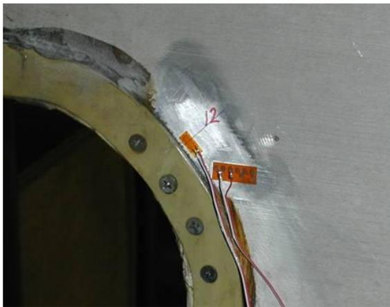
Figure 3. Door 5, Upper Corner Gauge Detail (1 gauge)
