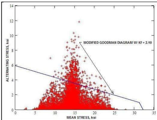
Figure 11. Modified Goodman Diagram with  $K_f = 2.10$
