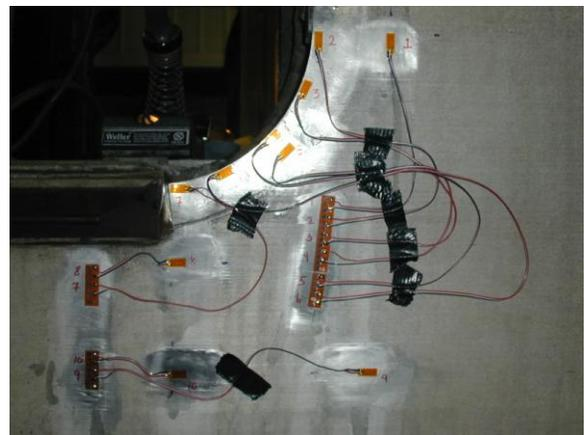
Figure 2. Door 5, Lower Corner Gauge Detail (11 gauges)
