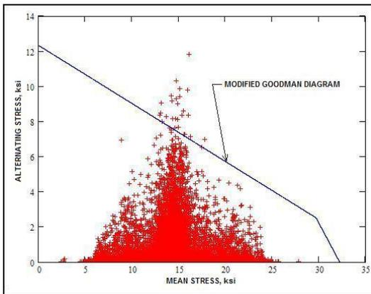
Figure 10. Modified Goodman Diagram with  $K_f = 1.00$
