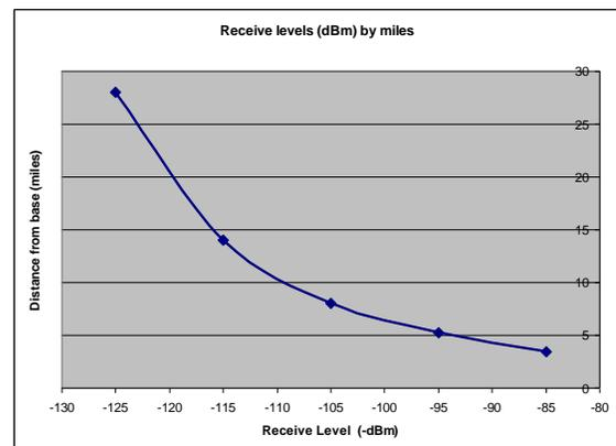
Fig. 4: Propagation output levels for 218 MHz Receive levels by Distance for BCP base test sites
