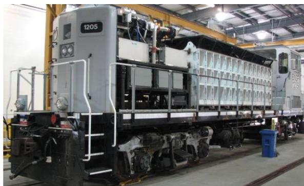
**Figure 2. Locomotive under construction:** Right-rear view of the locomotive with installed fuel-cell prime mover shown in the foreground (31 July 2008)
