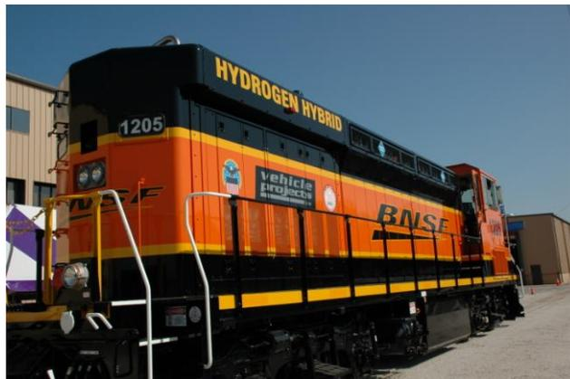
**Figure 1. Fuel-cell switch locomotive:** This is the largest fuel-cell land vehicle, photographed at a press conference in completed form on 29 June 2009
