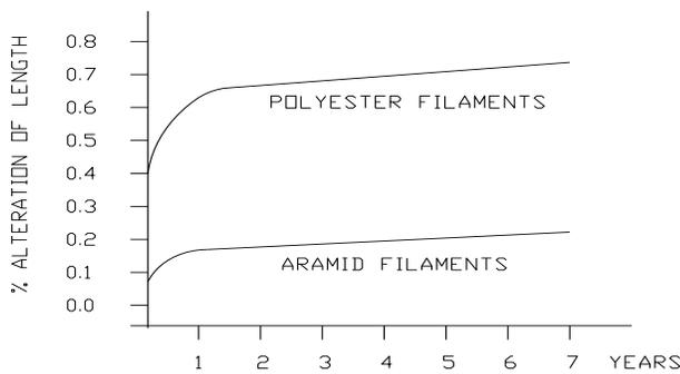
Figure 4. Long Term Test Results of Synthetic Rope
