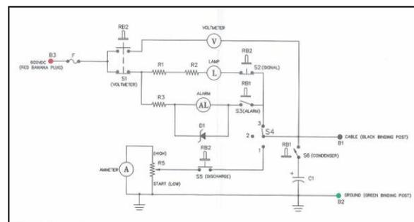
Figure 1. Test Set Schematic
