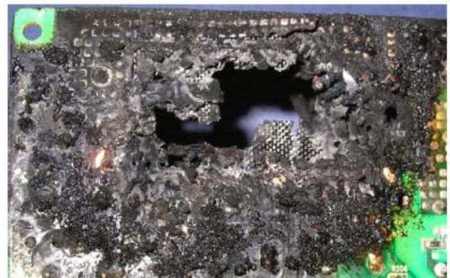
Figure 2- Damage from a Propagating PCB Fault (4)
