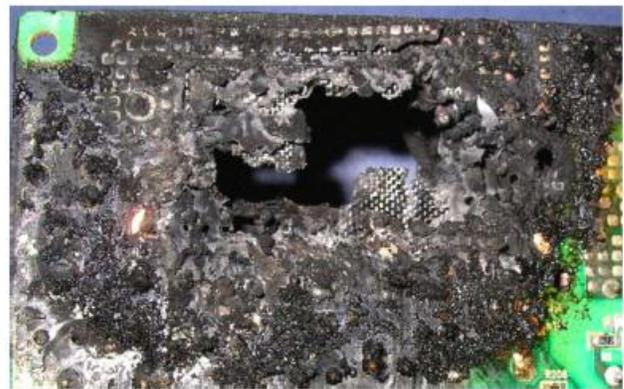
**Figure 2- Damage from a Propagating PCB Fault (4)**
