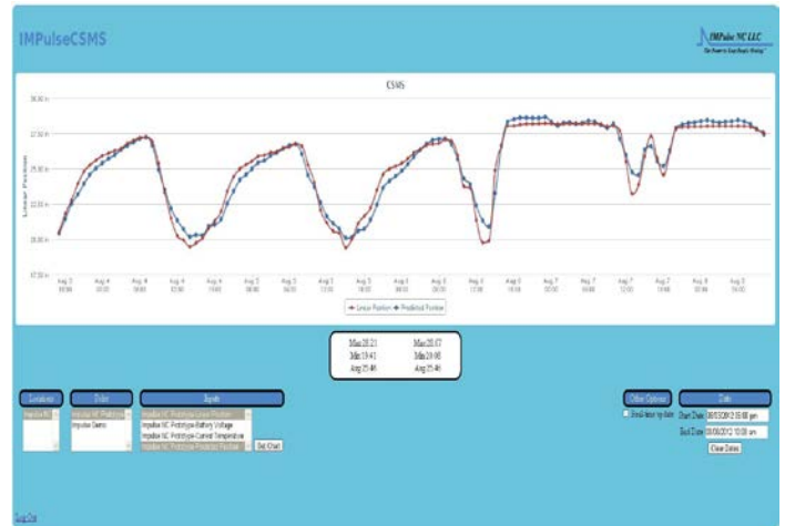
Figure 5 Real movement of properly working BWA compared to the predicted movement
