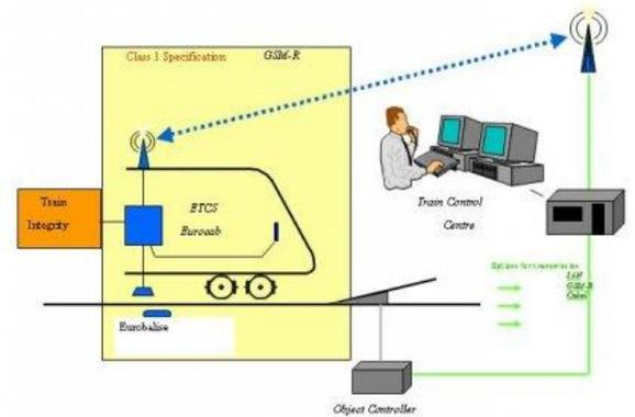
In theory, ERTMS level 2 would allow the removal of wayside signals as all the signaling information would be available onboard via a train driver display. It is noted, however, that ERTMS level 2 still uses the track circuits or axle counters for the train detection and for the train integrity monitoring function, unlike CBTC or ERTMS level 3 (see below).
