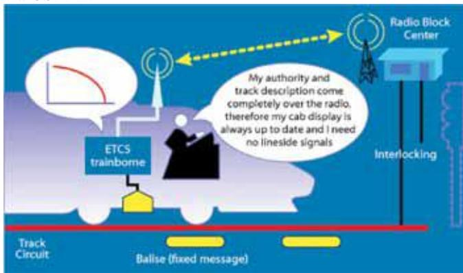
The full version of ERTMS Level 3 is still in the development phase and has not been implemented yet. However a variant of ERTMS Level 3 called “ERTMS Regional” has been implemented in Sweden for a low density line (Västerdal Line). In this case the main reason of this implementation was the reduction of O&M cost and safety improvement.
