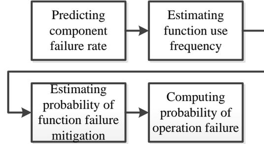
**Figure 1. Method for Estimating Passenger Operation Failure Probability**
