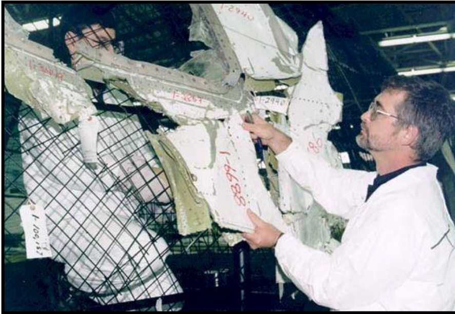
Wreckage reconstruction, Swissair
