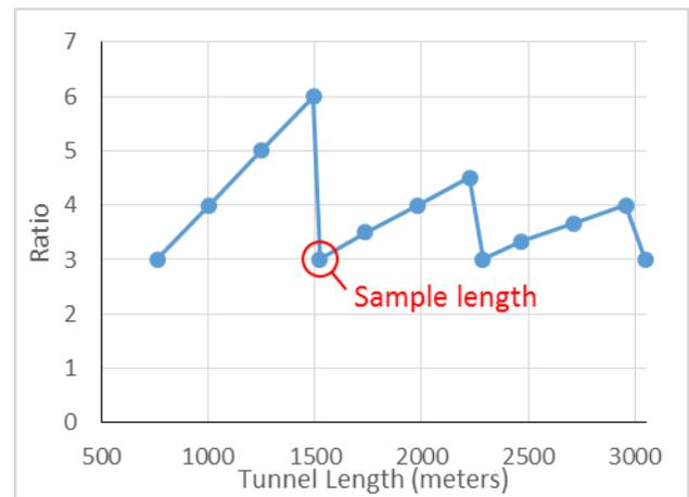
Figure 2: Ratio of Cross-passageways to Stairways vs. Tunnel Length
