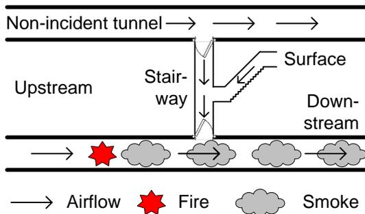
Figure 5: Airflow Prevents Smoke from Entering Stairway
