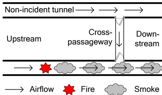
Figure 7: Airflow Prevents Smoke from Entering Cross-passageway
