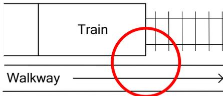
Figure 4: Egress Choke Point on Walkway after Train
