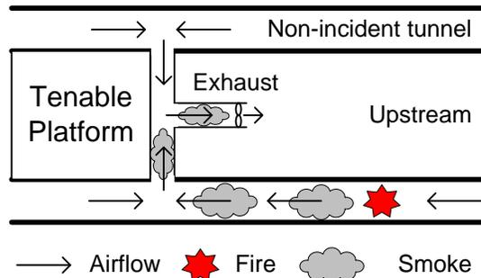
Figure 6: Airflow Creates a Tenable Platform
