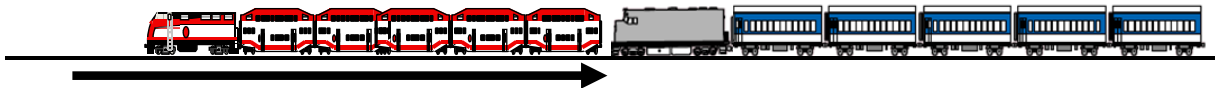
Figure 1: Train Level Collision Scenario with a cab car + 4 trailer cars and a locomotive
