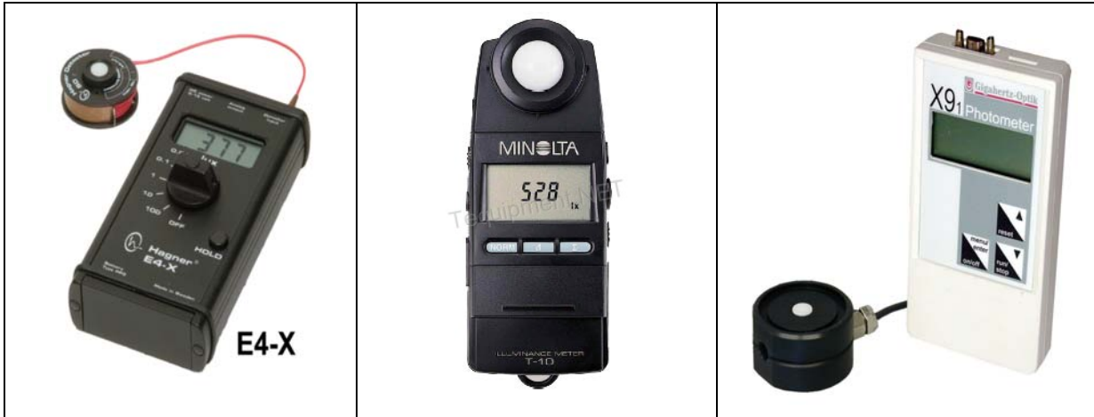
Figure C1. Typical meters for illuminance measurements
