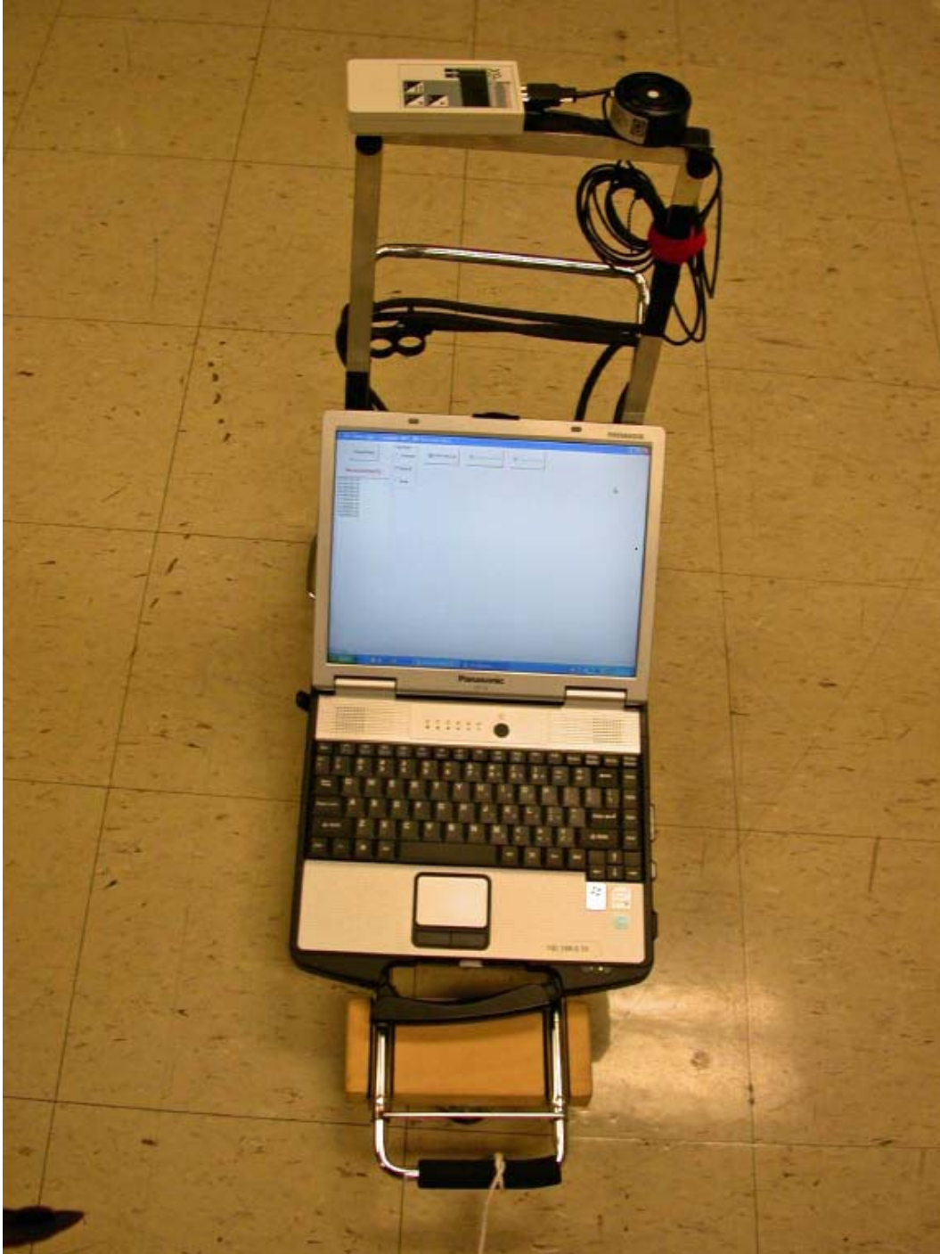
Figure C2. Apparatus for measuring average illuminance levels: Consists of a hand-held illuminance meter with sensor, an analog-to-digital converter (if not built into the meter), a notebook computer, a luggage cart with an added bracket to hold the sensor, an extra caster, and a towline.
