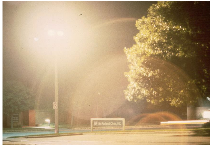
FIGURE 5 Impact of Glare on Visibility
