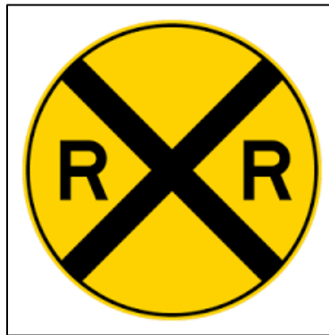
Figure 1: W10-1 Grade Crossing Advance Warning Sign
