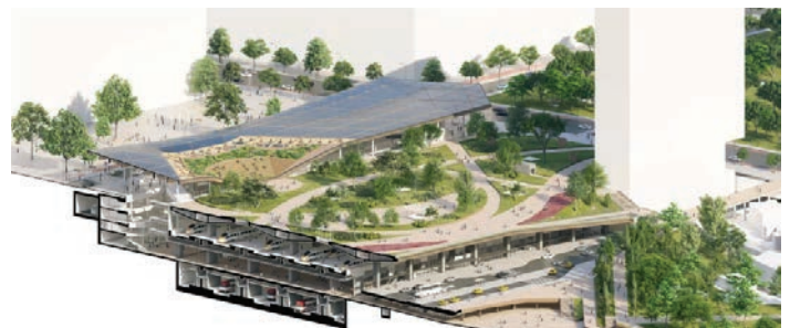
Figure 5- ^ Barcelona La Sagrera transforms an obsolete freight yard into a new mixed-income community linked by green space and transit. Rail and roads will be placed below grade, while new parkland will be created above the tracks. The station gives the future 180,000 residents who will live in this vicinity direct access to new open space while removing physical barriers to circulation.
