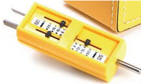
FIGURE 7 Outlet Tension Tester
