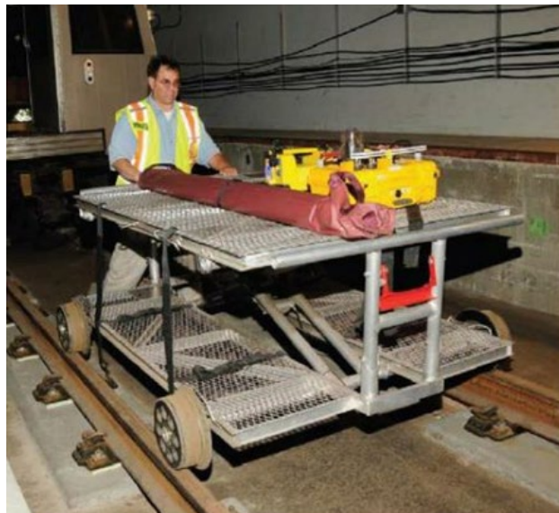
FIGURE 1 WMATA's Emergency Tunnel Evacuation Cart
