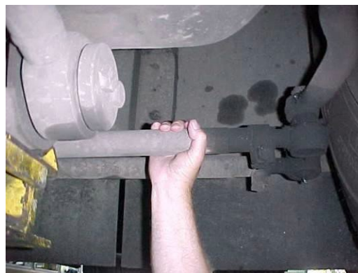
FIGURE 6 Checking Tie Rod Ends
