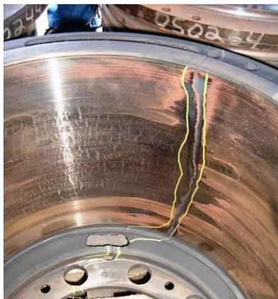
Cracked brake drum
