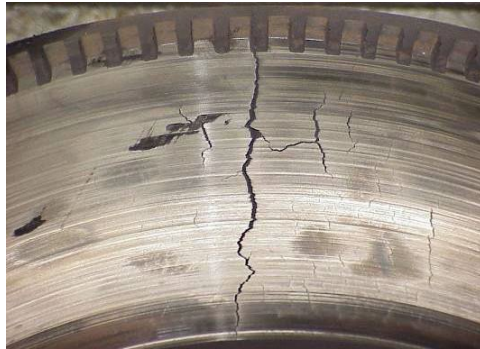
Excessive drum crack
