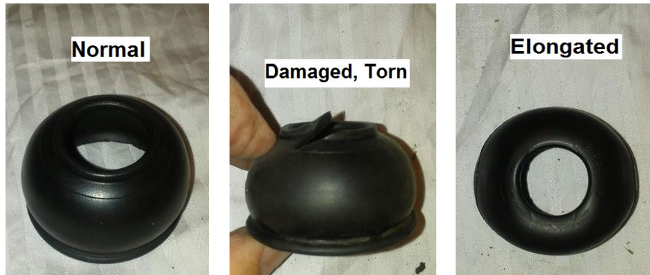
FIGURE 3 Rubber Boot Wear
