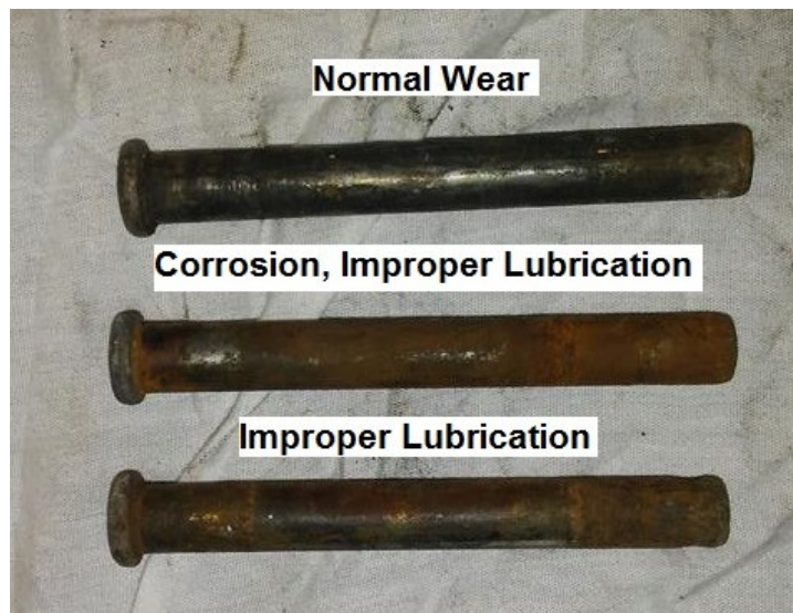
FIGURE 2 Pivot Pin Wear
