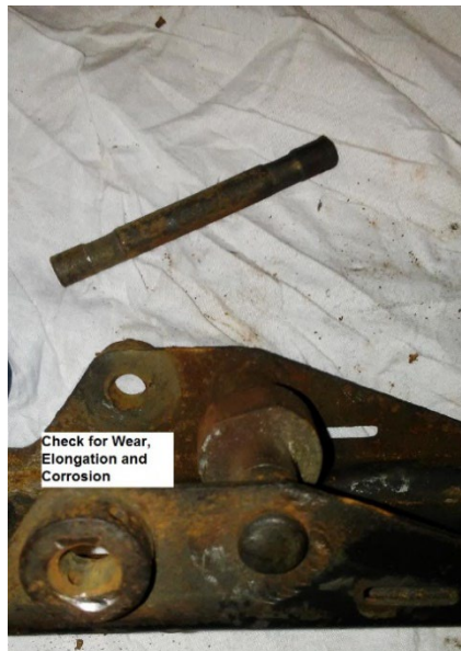
FIGURE 8 Roller and Pin Wear
