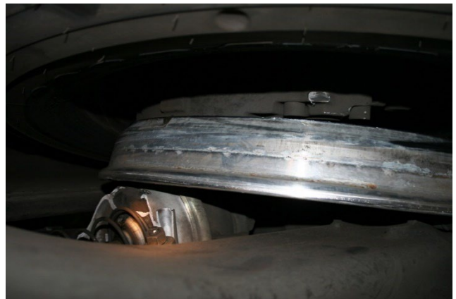
Damaged rim and brake chamber caused by a missing pad retainer strap
