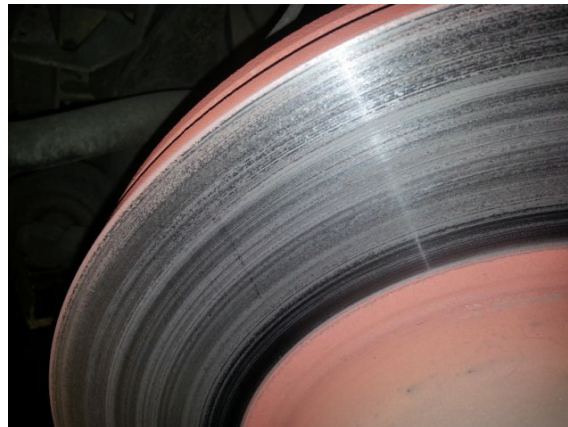
FIGURE 42 Evidence of Overheating
