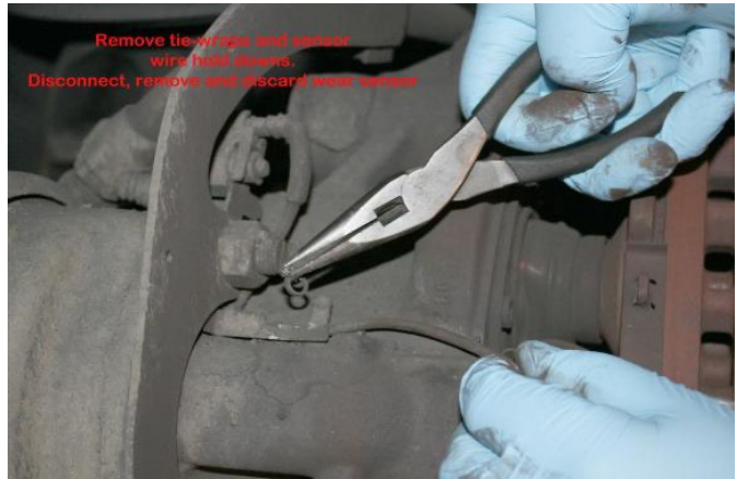
Remove in-pad sensor components if so equipped
