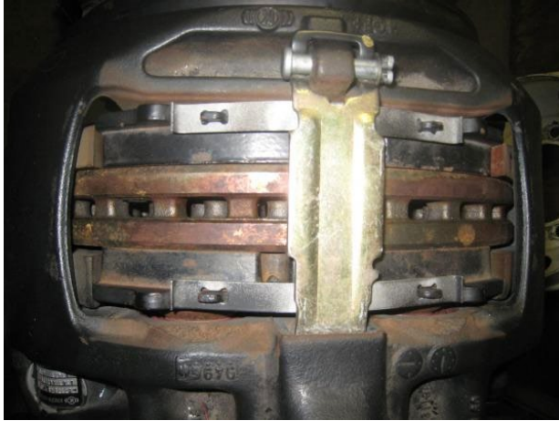
Knorr-Bremse pad retainer with clevis pin
