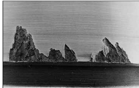
Geometric Stress Concentration (GSC) spalling
