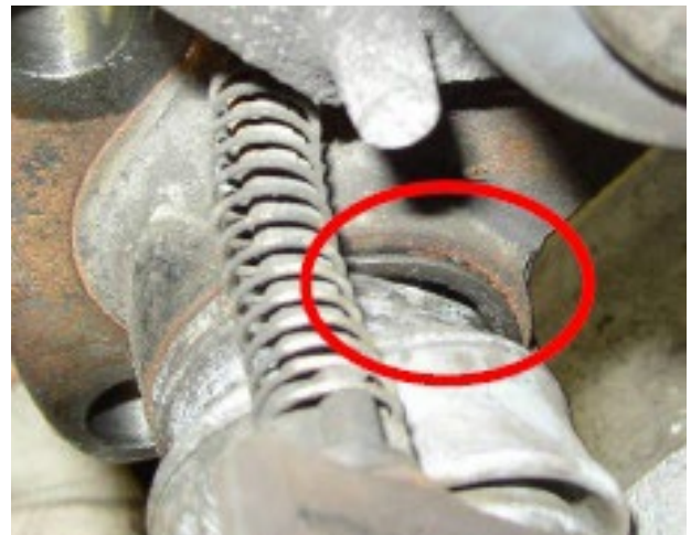
Improperly installed slide pin boot
