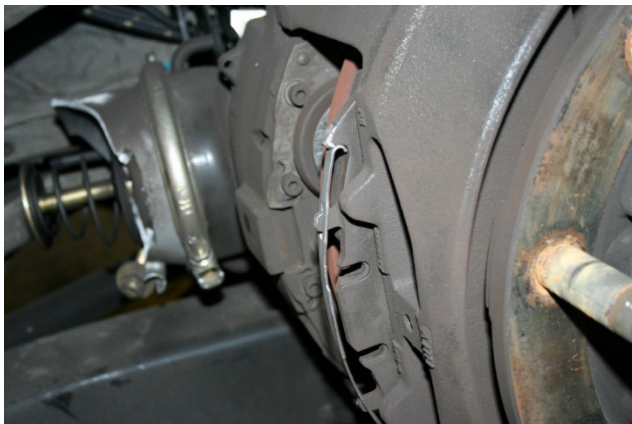
Damage caused by a missing pad retainer strap
