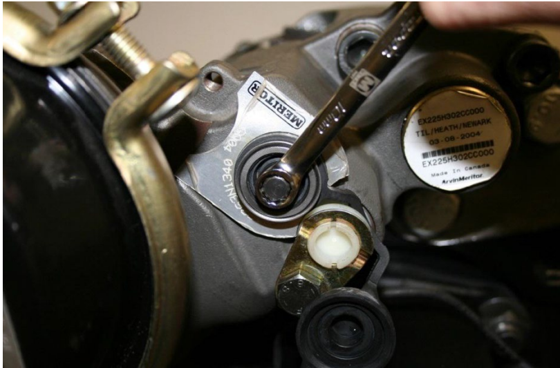
FIGURE 28 Checking Meritor EX225 Adjuster
