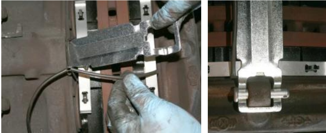
Knorr-Bremse pad retainer installation
