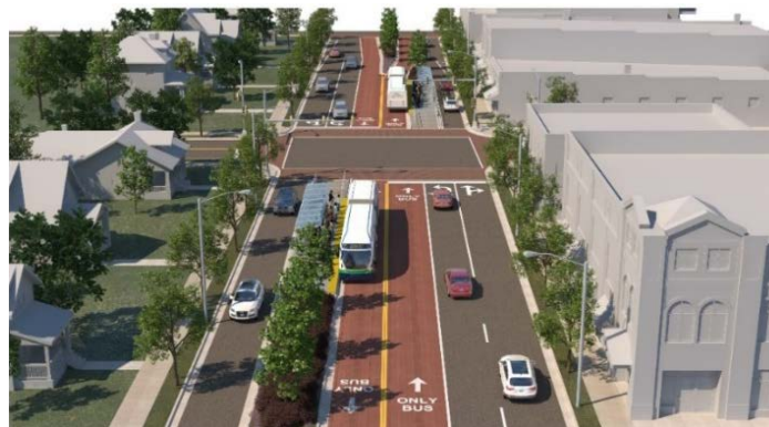
Median Busway with Offset Stations for Right Side Boardings
