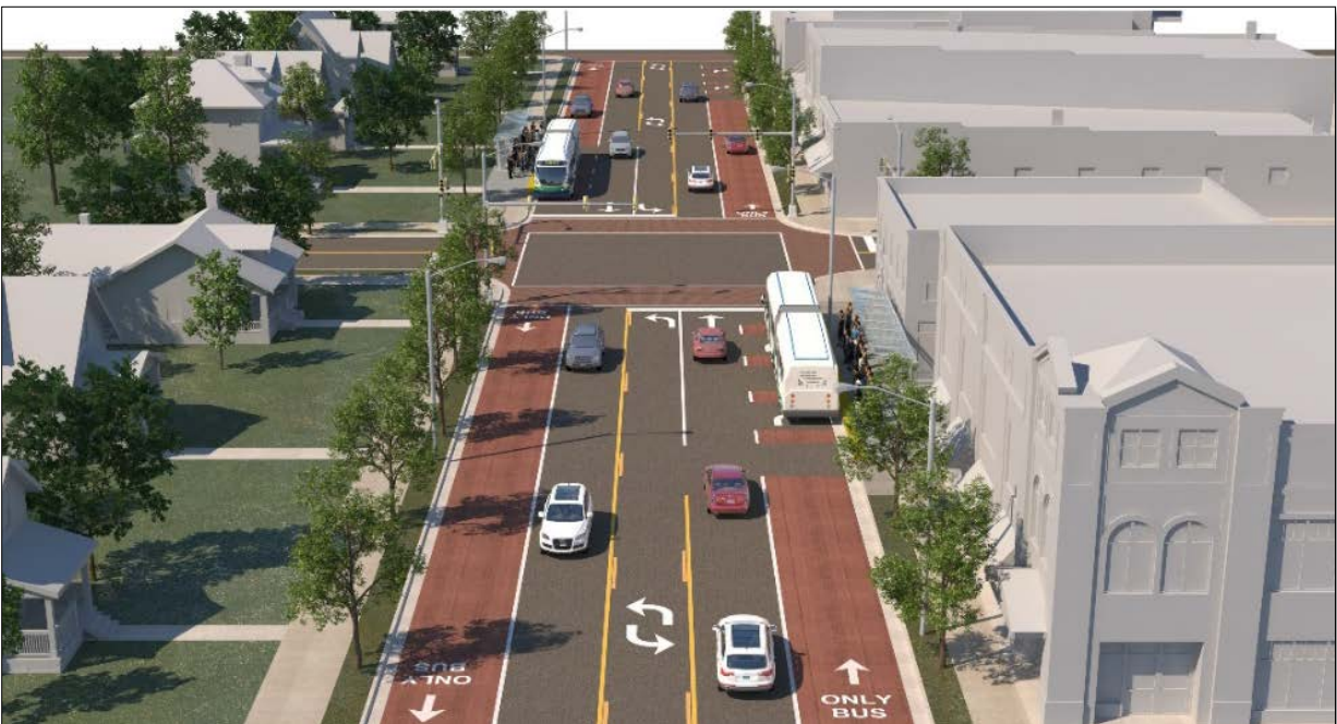
FIGURE 18 BAT Lane with Near Side Stations
