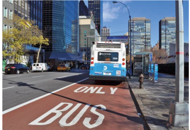
FIGURE 3 Arterial BRT Running Ways
