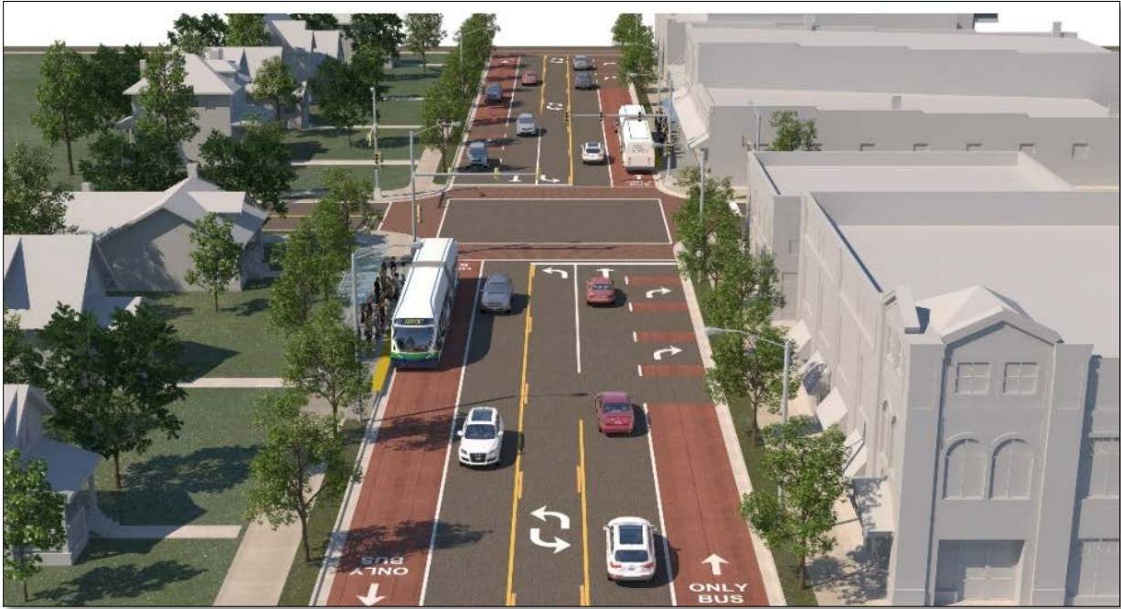
FIGURE 18 BAT Lane with Near Side Stations
