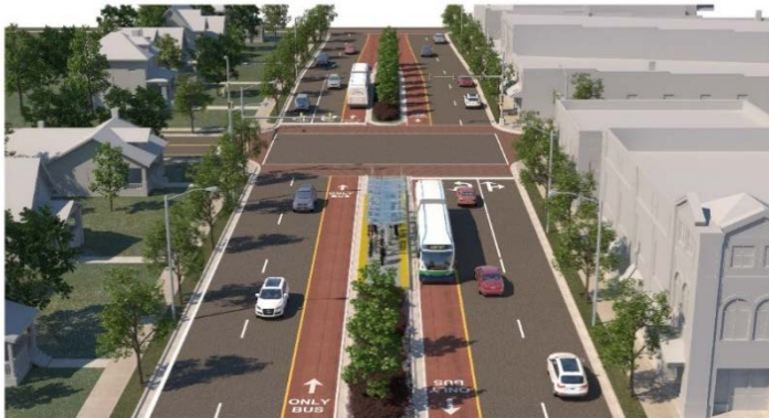
Median Busway with Center Station, Counter Flow for Right Side Boardings
