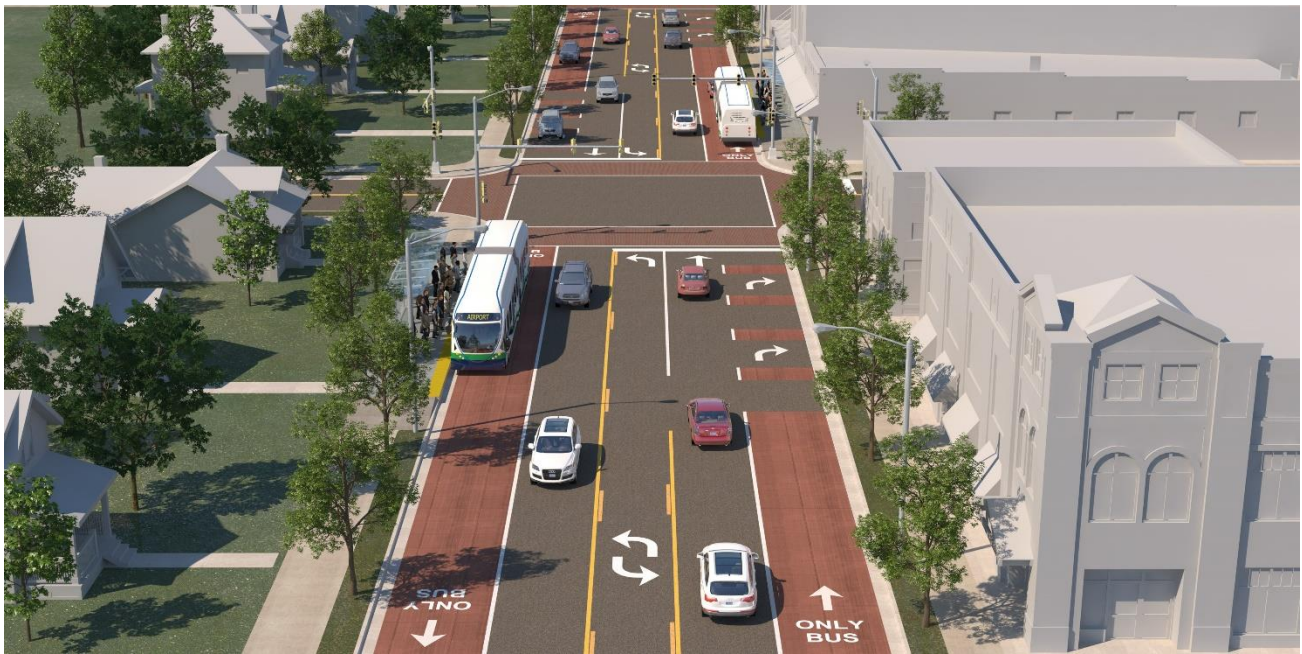
FIGURE 7 BAT Lane with Striping
