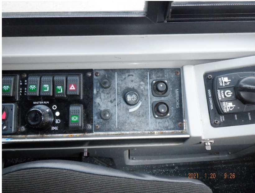
Figure 1 Surface degradation caused by pesticide disinfectants
