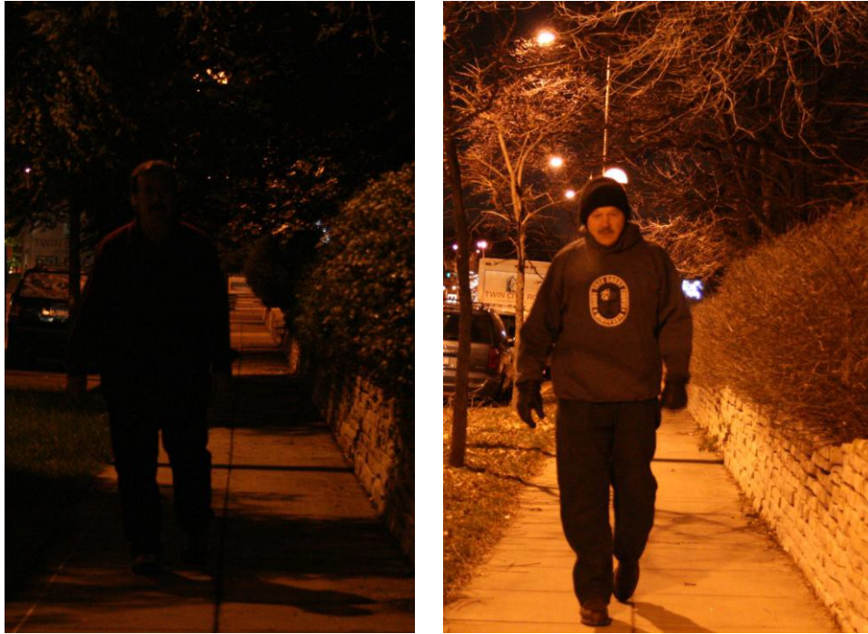
FIGURE 6 Impact of Vegetation on Lighting Systems
