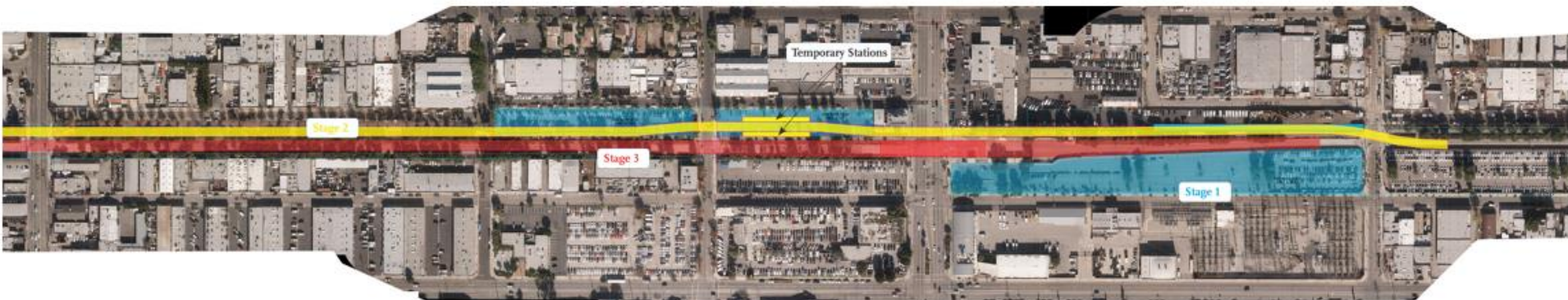
Figure 3-3: Construction Staging (Van Nuys Station)
