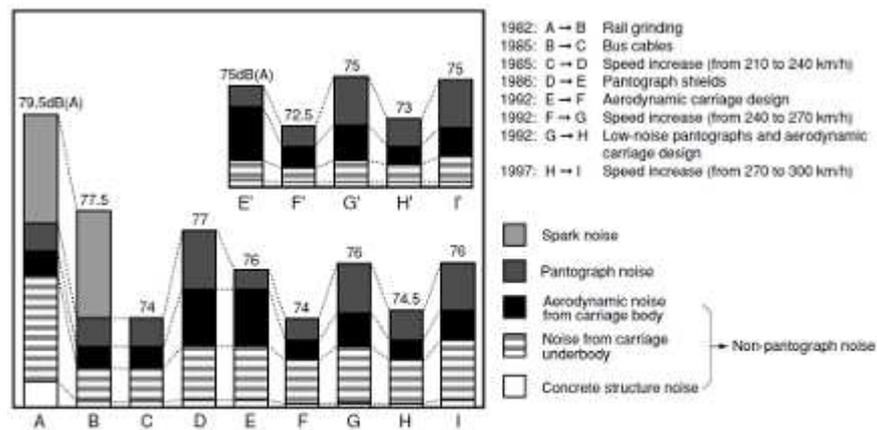
Measured at ground level, 25 m from concrete elevated track, 8 to 10 m from ground level to rail level with slab track.
