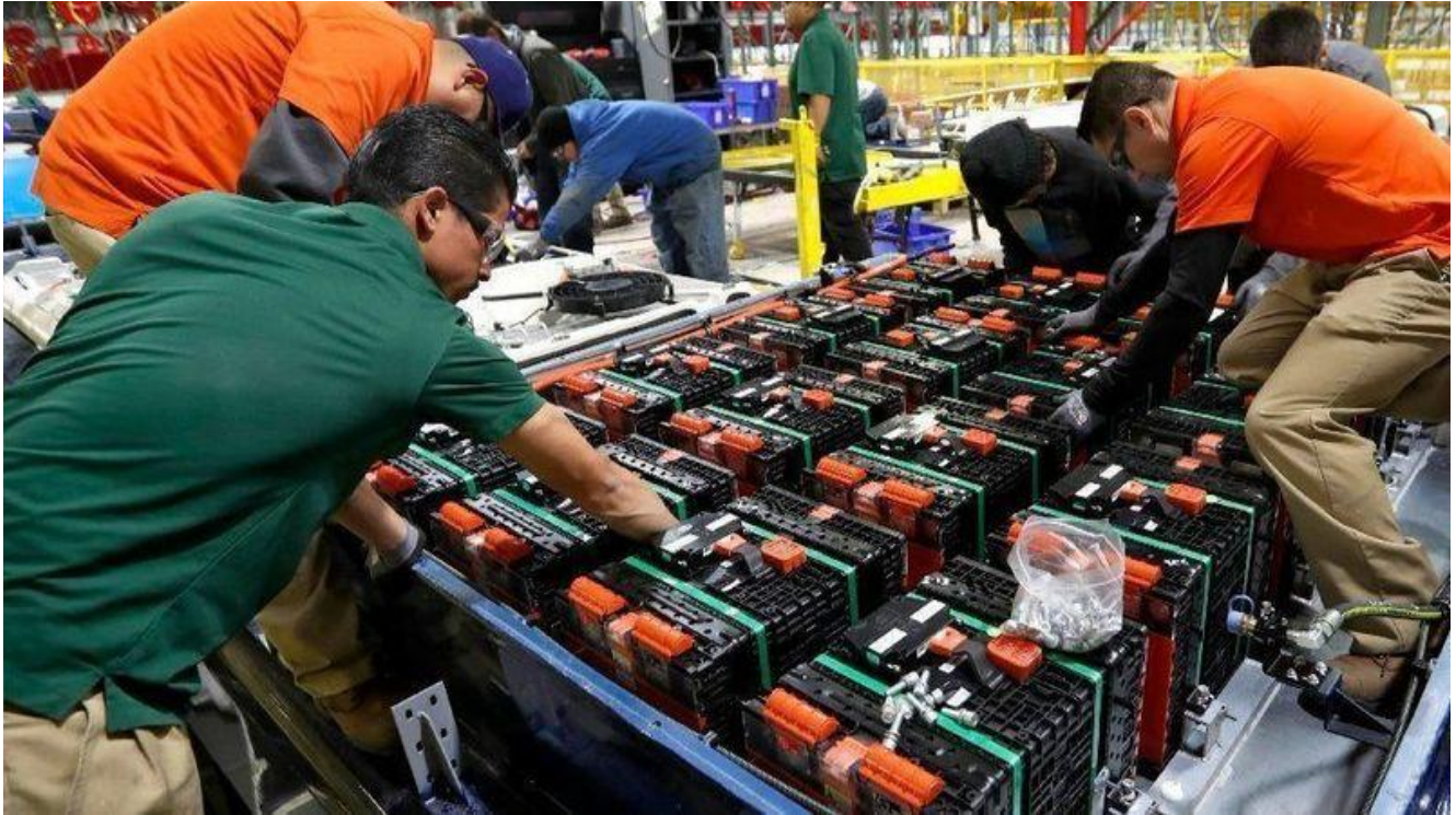
Workers install batteries on top of a bus destined for UC Irvine. BYD's business began with production of cellphone batteries. (Mel Melcon / Los Angeles Times)
