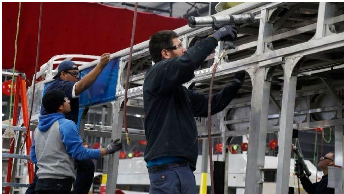
BYD assembly plant worker Jesus Martin applies glue before an aluminum skin is placed on the exterior of an electric bus at the BYD production facility in Lancaster. (Mel Melcon / Los Angeles Times)
