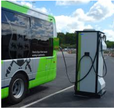
Electric Bus Depot Chargers 23 kW x 2000 “plug-in”
