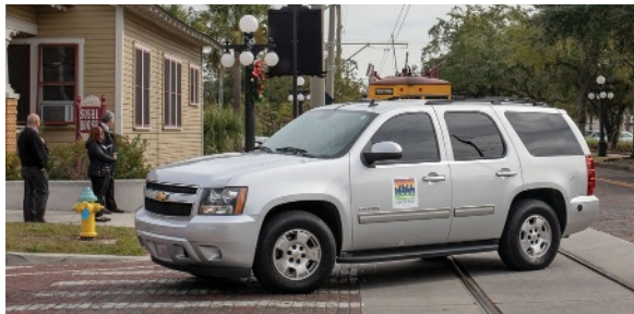
As part of a connected vehicle pilot program in Tampa, FL, two connected vehicles—a TECO Streetcar and a car—receive warnings when the car pulls in front of the moving streetcar.
