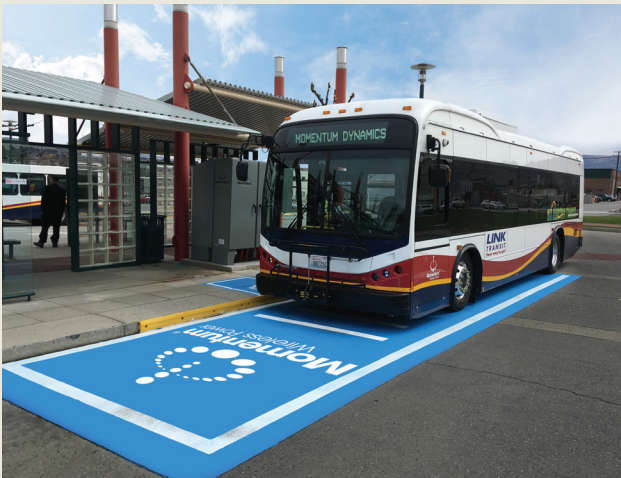
A Momentum Dynamics wirelessly charged Link Transit bus.
