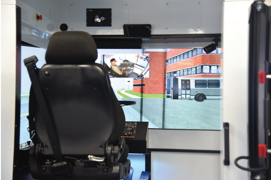
With VTA's new MB-2000 bus simulator, the cab can be configured to match the layout of controls, indicators, gauges and switches of the agency's fleet vehicles.
