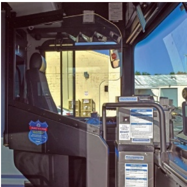
The driver safety shield installed in a HART bus.
