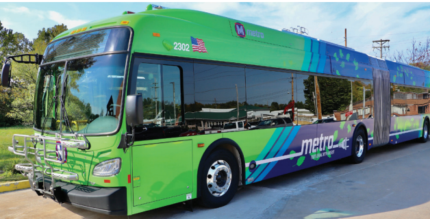
Each of Metro Transit’s new 60-foot battery electric buses have 320 kilowatts of battery storage—enough to power 10 2,000-square-foot houses for an entire day.
