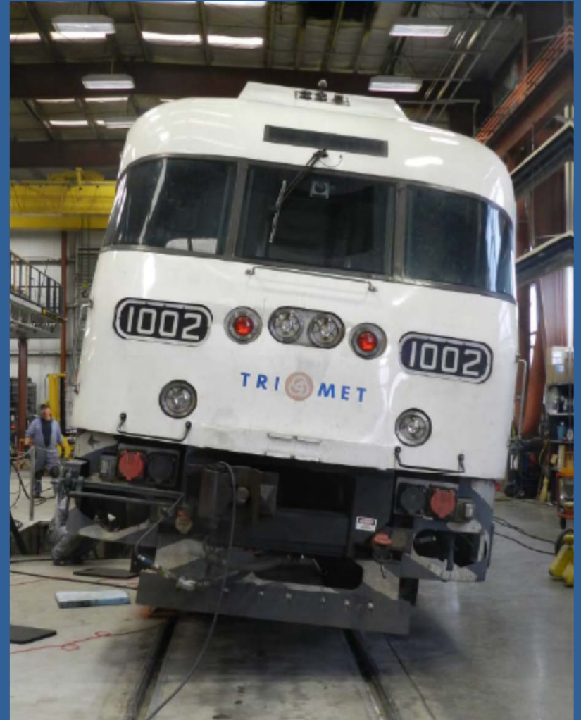
Car 1002 at 6" Superelevation
