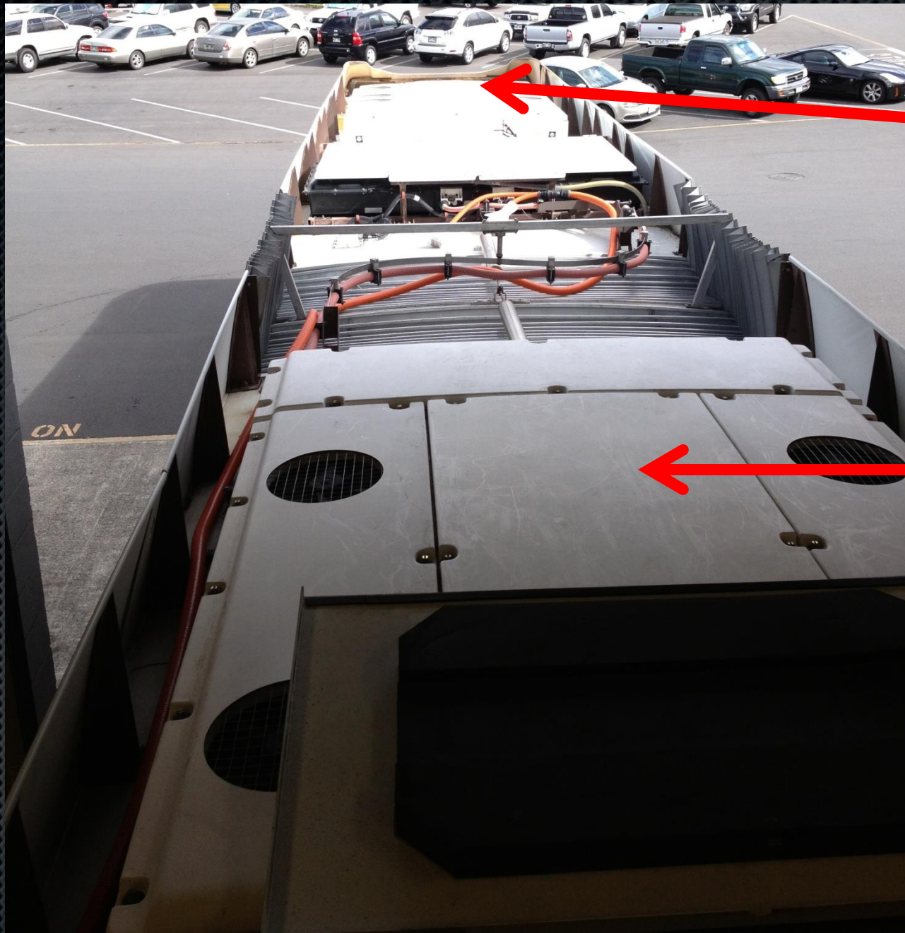
Dual Sutrak Fully-Electric A/C on roof and getting power from HVDM
