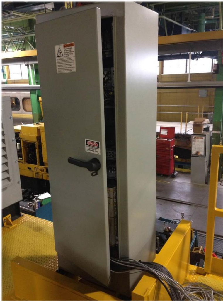
ATP Enclosure and on-board controller
