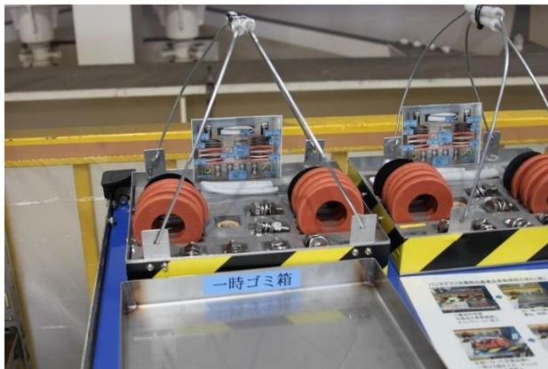
As an example, materials for Preventive Maintenance are staged on the carts identified by the car number ready for the car to roll into the shop.
