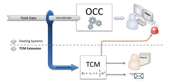
The Track Circuit Monitoring Tool utilizes track circuit status information and analyzes this information – in real time – to detect irregular operation and potentially unsafe conditions. TCM separates and alerts only those conditions, creating potentially unsafe conditions and affecting the reliability and of rail systems.
