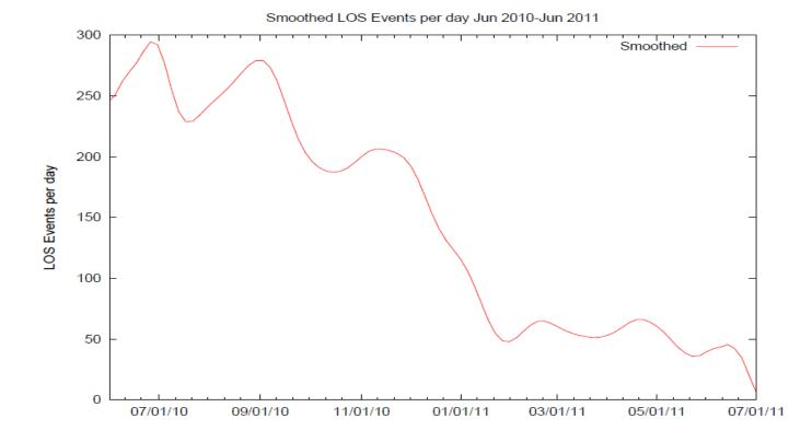
As the tool was refined and the review process between Engineering and Maintenance was applied, the number of alarm events continuously fell from a high of almost 300 per day to about 10 per day over the period July 2010 to July 2011.
