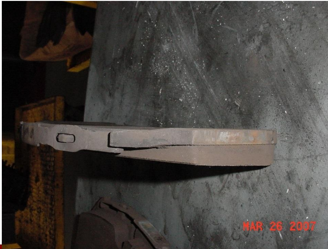
Brake pad uneven wear (taper)
