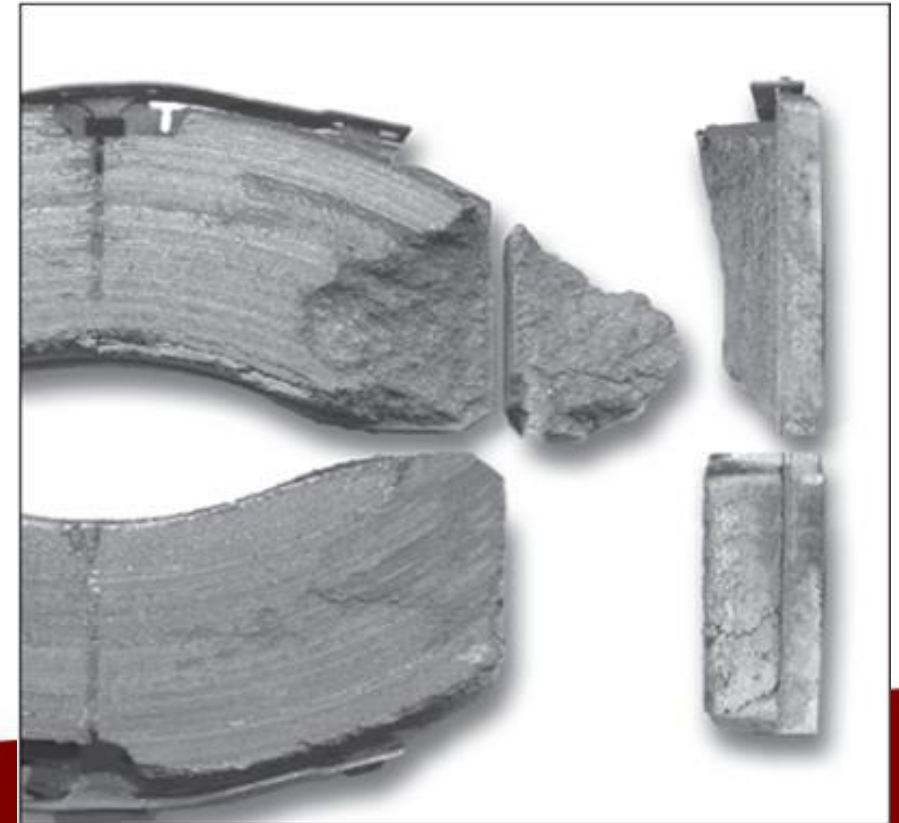
Brake pads showing unacceptable wear—note edges
