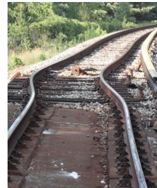
Figure 2: DC Metro Heat Kink, July 2012 Heat wave
