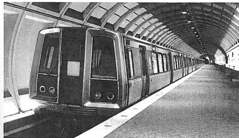
Modern rail station design minimizes crime by eliminating columns, dark corners, and other areas where criminals can lurk. This Washington Metropolitan Area Transit Authority heavy rail station illustrates such design.
