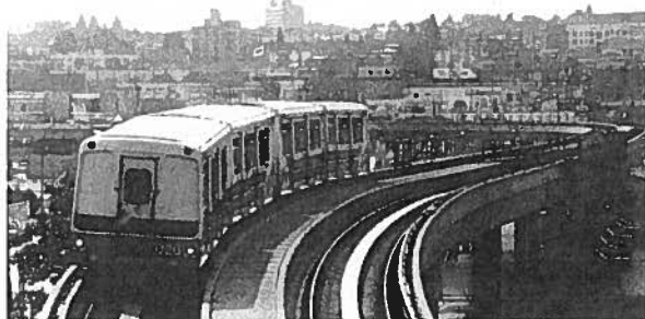
North America's longest driverless automated rail system—nearly 18 miles long—is SkyTrain of Vancouver, British Columbia.
