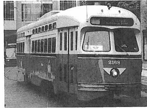
The Presidents' Conference Committee (PCC) car was the industry's concerted attempt in the 1930s to standardize and modernize the numerous streetcar designs and win back riders. The Southeastern Pennsylvania Transportation Authority in Philadelphia operated this one.
