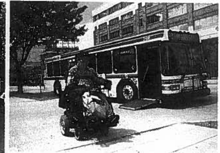
The wheelchair ramp is clearly visible on this Transit Authority of River City low-floor bus in Louisville, Kentucky.
