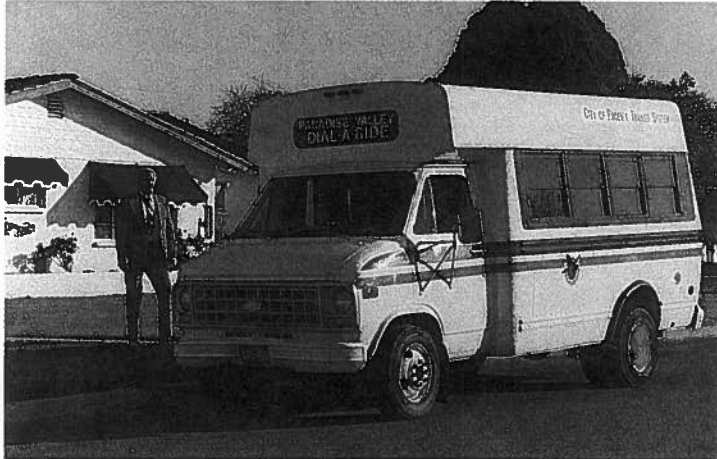
A typical body-on-chassis van operated by Arizona's City of Phoenix Transit System.
