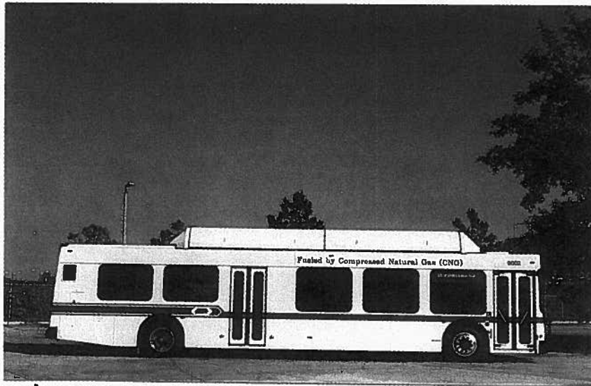
This bus is powered by the most popular alternative power, compressed natural gas. Due to the low-floor configuration, the CNG tanks are located on the roof of the bus. The Pinellas Suncoast Transit Authority that serves the St. Petersburg, Florida area is the operator of this bus.
