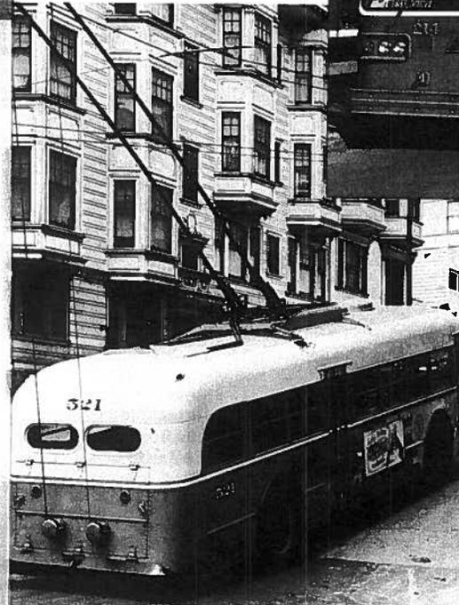
Electric rubber-tired trolley coaches (trackless trolleys) solved a common problem of many street railway companies which desired to remove deteriorated, expensive-to-maintain tracks while retaining inexpensive electricity to power vehicles. San Francisco Municipal Railway Coach No. 521 was delivered in 1947 by the St. Louis Car Co. during the peak period of trolley coach construction; between 1930 and 1952 over 8,000 trolley coaches were delivered to U.S. transit systems.
