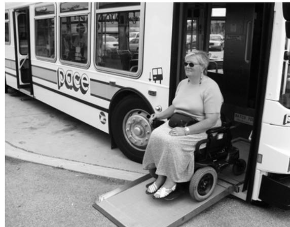
*This Pace bus, which services the suburbs of Chicago, Illinois, has a low floor and is equipped with a ramp.*
