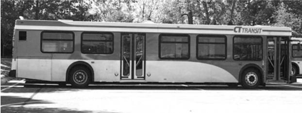
Connecticut Transit operates this 40-foot-long bus, the most common, in both Hartford and Stamford Connecticut. Most buses are high-floor models having two or three steps, but this is a low-floor model without steps.
