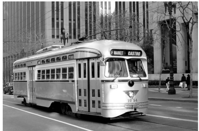
*This San Francisco Municipal Railway light rail vehicle is powered by overhead electrical wires.*
