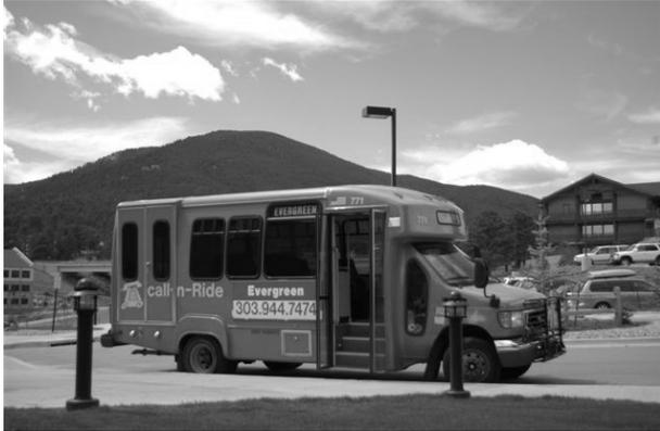
A typical body-on-chassis van operated by the Regional Transportation District in Denver, Colorado. Although this particular van is being used for demand response service, this type of vehicle is often used for lightly-patronized fixed route service.
