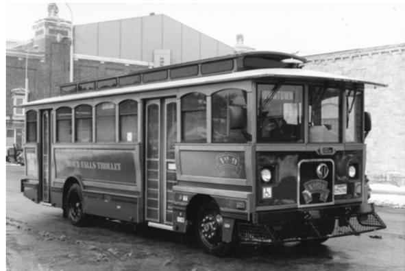
Often called a trolley, this vehicle that imitates an old streetcar is called a "trolley replica bus." Its data are included with bus statistics since it is rubber-tired and has an on-board power source. This is a Sioux Falls Transit vehicle in City of Sioux Falls, South Dakota.
