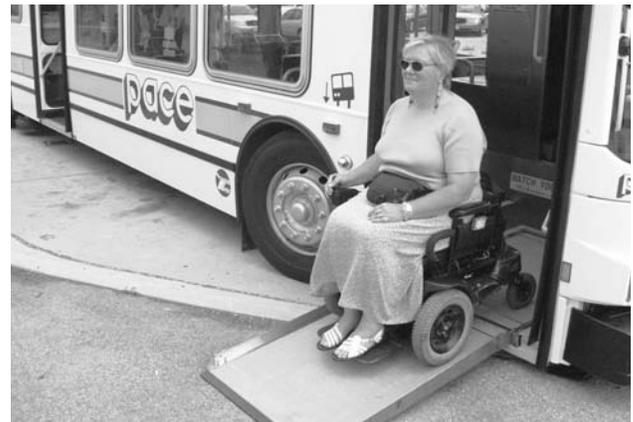
*This Pace bus, which services the suburbs of Chicago, Illinois, has a low floor and is equipped with a ramp.*
