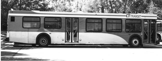
Connecticut Transit operates this 40-foot-long bus, the most common, in both Hartford and Stamford Connecticut. Most buses are high-floor models having two or three steps, but this is a low-floor model without steps.
