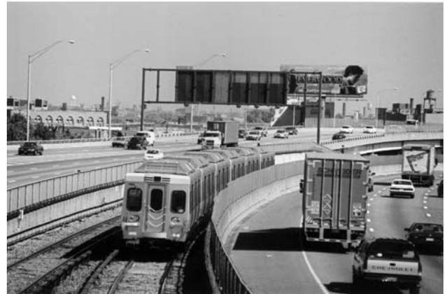
*A Southeastern Pennsylvania Transportation Authority train in Philadelphia, Pennsylvania, operates in a freeway median. When counting vehicle miles and hours for trains, each car is counted, so this 6-car train operates 6 vehicle miles for each mile traveled and 6 vehicle hours for each hour in service.*
