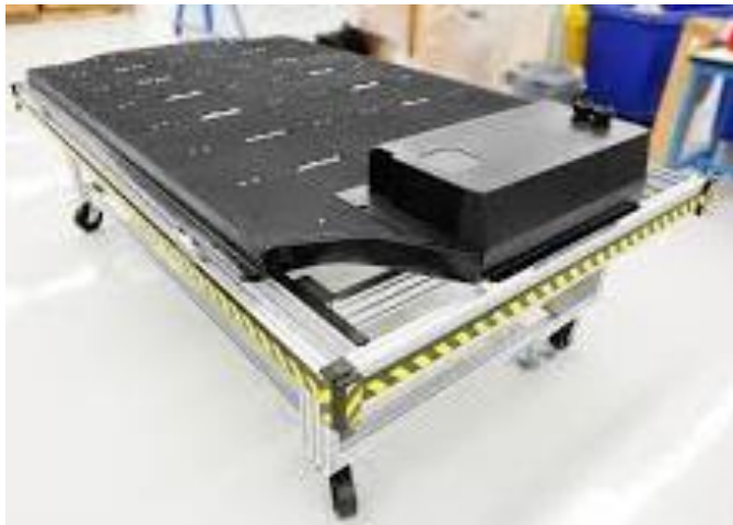
Model S liquid cooled battery pack
