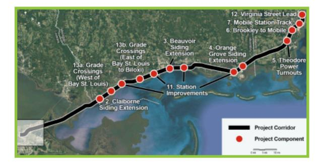
of intercity passenger rail while maintaining freight service reliability along the Gulf Coast. The improvements would include lengthening passing sidings to allow for longer freight trains, extending main tracks, installing new switches and turnouts, constructing additional crossovers, and improving stations, yards, and grade crossings. The estimated cost of the program of projects is \$223 million.
