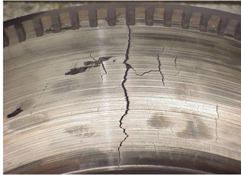
Excessive drum crack
