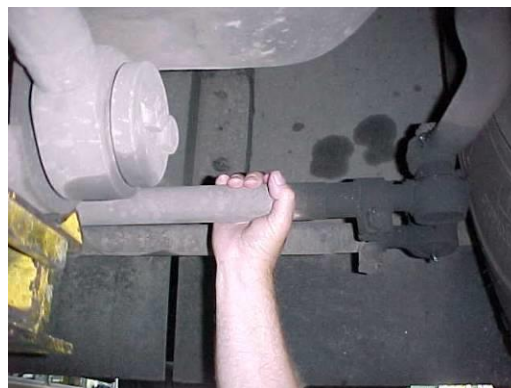
FIGURE 6 Checking Tie Rod Ends
