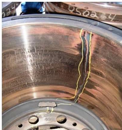
Cracked brake drum
